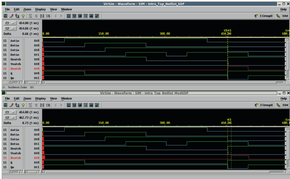
Fig. 23-4. Back-annotated netlist timing: Original SDF (above) vs. hand-modified SDF.
