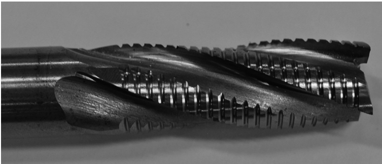
Fig. 3.16 Trapezoidal cutter showing the form of the cutting edge
