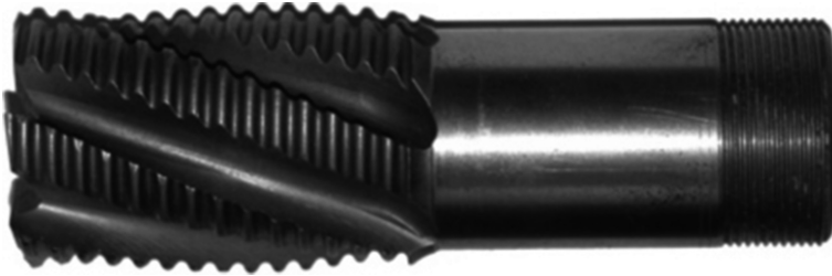
Fig. 3.9 Strasman (or roughing/ripping) cutter showing the sinusoidal form of the cutting edge
