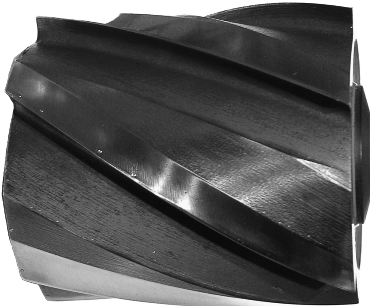
Fig. 3.39 Bi-helix slab mill with alternating 25° and 35° helices
