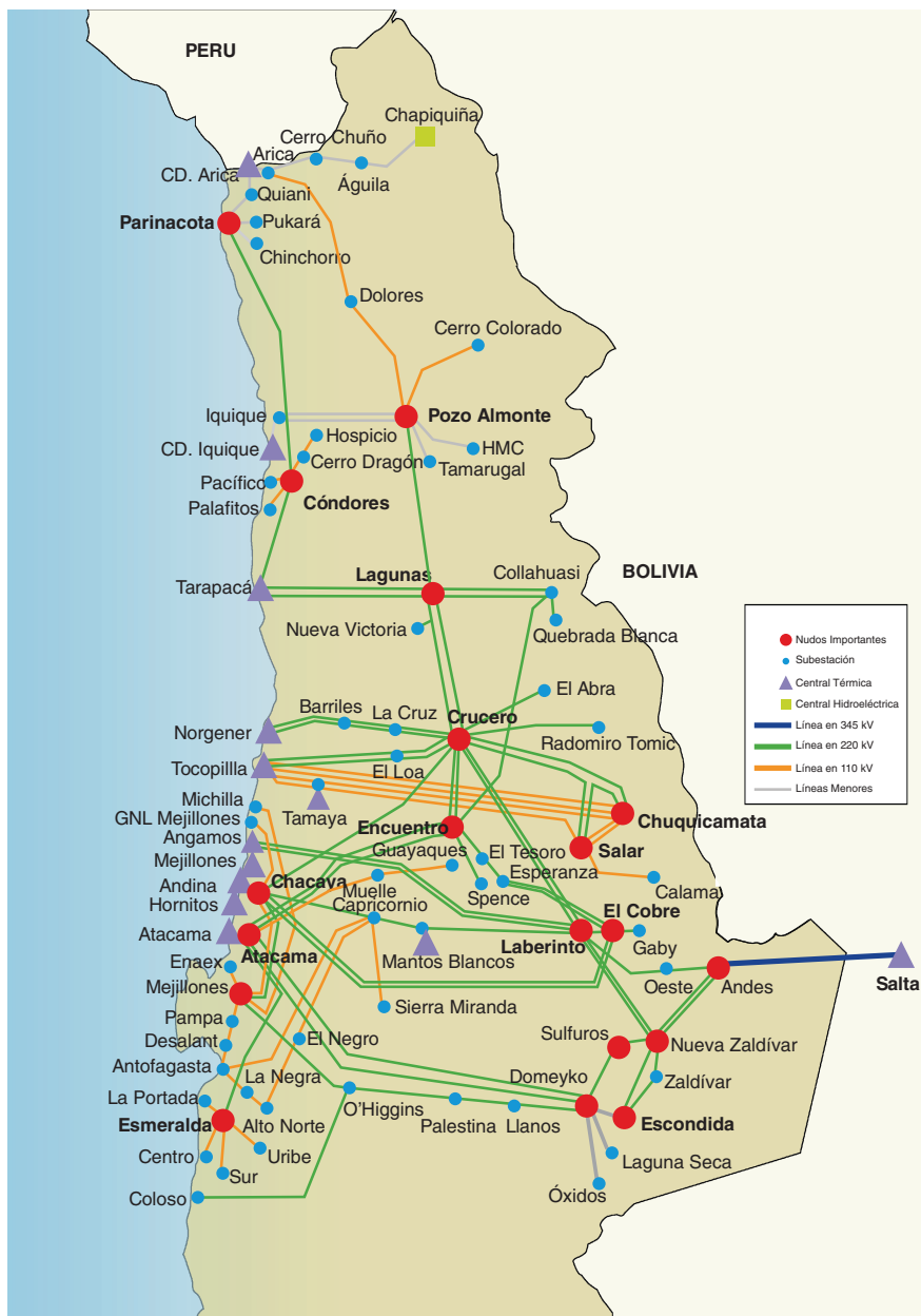
Fig. 10.3 One-line diagram of the SING
