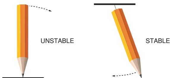
Fig. 9.1 Unstable and stable configurations for a pencil
