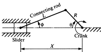
The figure shows the slider crank mechanism as used in the petrol and diesel engine as well as in reciprocating pumps and compressors. There are hundreds of millions of such mechanisms throughout the world. As it is a very important device we propose to examine its kinematics.
