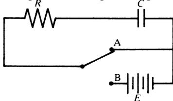
The figure shows a simple circuit consisting of a capacitor of  $C$  farads, a resistor of  $R$  ohms, two switches A and B and a battery having a constant voltage  $E$ .
