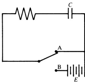
Case (b): Referring to the diagram, if the charge is  $Q_0$  when  $t = 0$  and switch  $A$  is closed ( $B$  open) a current will flow in the circuit and the capacitor will discharge.
