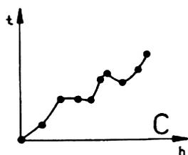
This curve represents all measured values, but it would not be chosen by physicists or engineers. We know that the accuracy of measurements depends on the used instruments and we always have errors in measurements. In our case we assume that the time of fall increases with the height of fall. Thus, we prefer curve B as the best fitting curve and regard the deviations from the fitting curve as errors of measurement. In chapter 21 “Theory of errors” we will discuss this topic again.
