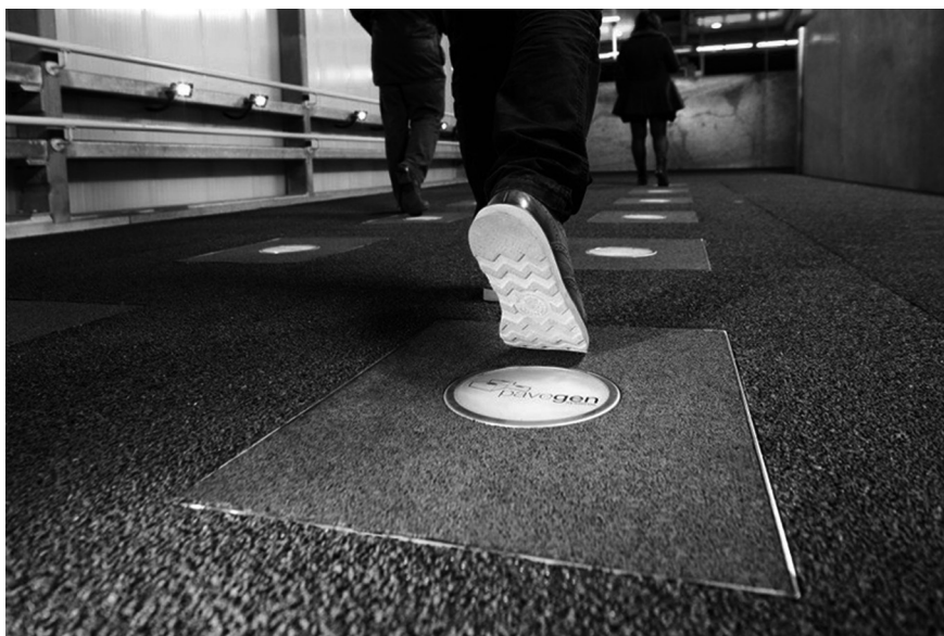
Fig. 18.13 Pavegen: kinetic energy generation from footsteps (Pavegen 2012)
