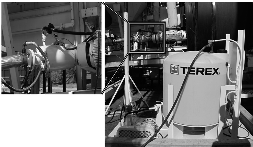
Fig. 10.6 Warm Mix Asphalt System water tank with water pump (right) and foam expansion chamber (left)
