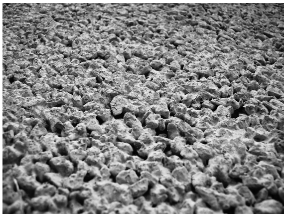
Fig. 8.4 Pervious concrete surface texture
