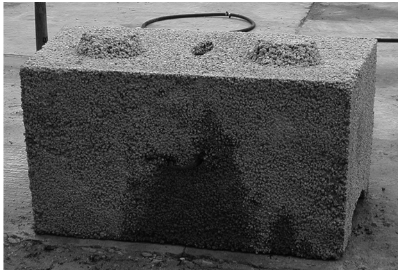
Fig. 8.10 Pervious concrete retaining wall block
