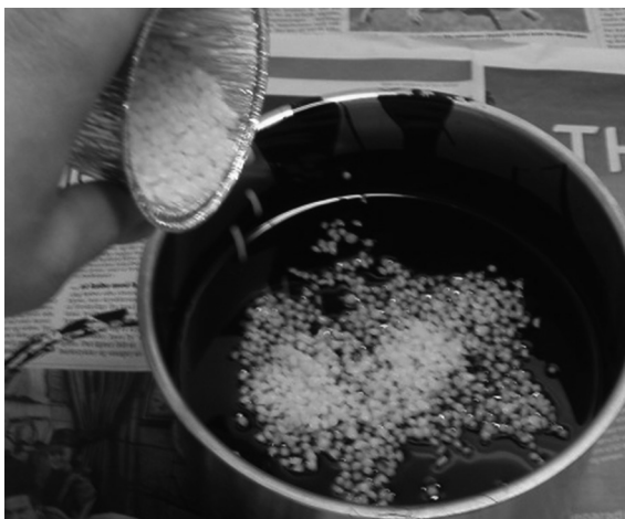
Fig. 10.8 Sasobit addition to binder in laboratory
