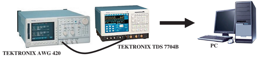
Fig. 13.8 WER measurement setup
