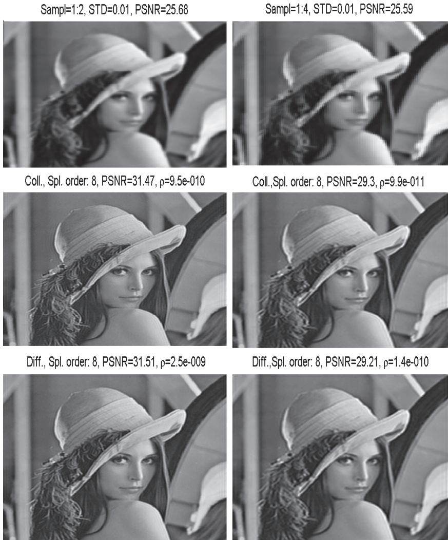
Fig. 7.17 Top left the blurred “Lena” image downsampled at 1:2, noise STD is 0.01, PSNR = 25.68 dB. Top right the image downsampled at 1:4, PSNR = 25.59 dB. Center the eight-order inversion splines designed by the collocation . Left sampling 1:2, PSNR = 31.47 dB. Right sampling 1:4, PSNR = 29.3 dB. Bottom eight-order inversion splines constructed by the difference . Left —sampling 1:2, PSNR = 31.51 dB; Right sampling 1:4, PSNR = 29.21 dB
