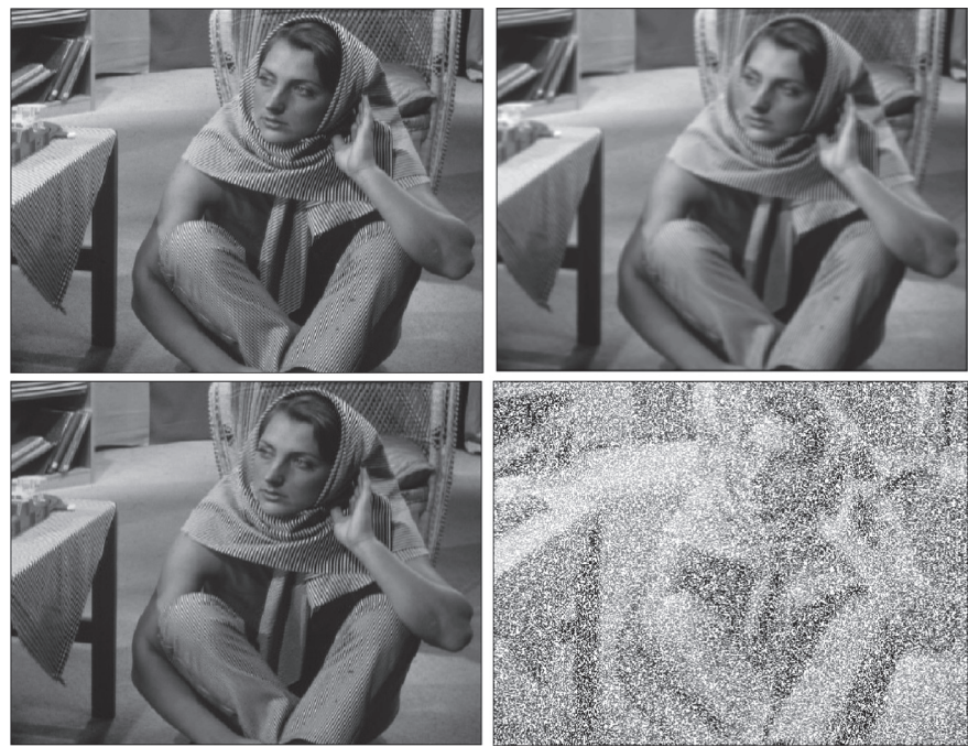
Fig. 18.6 Top left Source input—“Barbara” image. Top right Blurred, PSNR = 23.32 dB. Bottom right After random removal of 50 % of its pixels. PSNR = 9.34 dB. Bottom left The image restored by the frame T^4_{100,0} . PSNR = 30.32 dB
