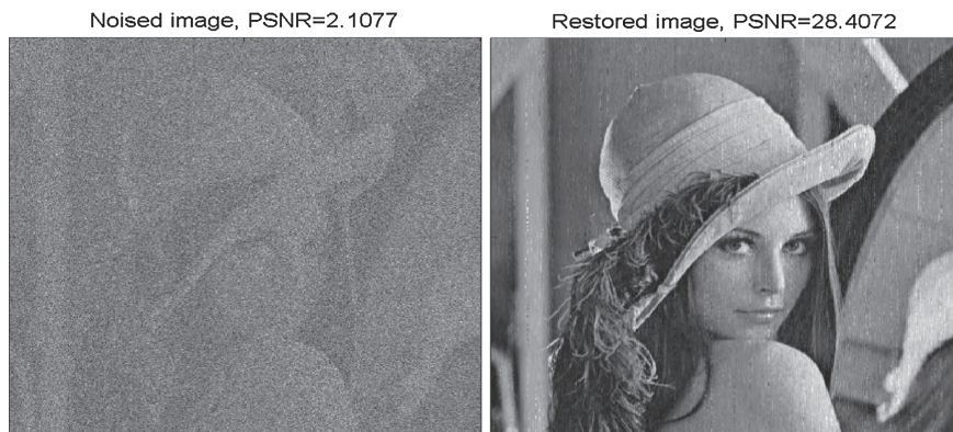
Fig. 14.27 Dummy example: reconstruction of the “Lena” image from a noised ( \text{STD} = 200 ) input. Left input; Right restored image
