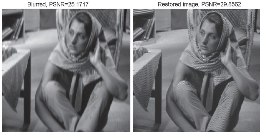
Fig. 10.9 Reconstruction of the “Barbara” image from a blurred (Gaussian, \sigma = 3 ) input
