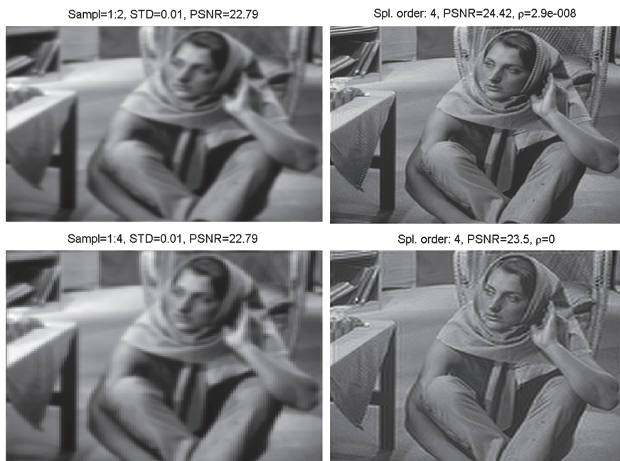
Fig. 7.12 Top left the blurred "Barbara" image downsampled at 1:2, noise STD is 0.01, PSNR = 22.79 dB. Top right the cubic deconvolution spline, PSNR = 24.42 dB. Bottom left the image downsampled at 1:4, PSNR = 22.79 dB. Bottom right the cubic deconvolution spline, PSNR = 23.5 dB
