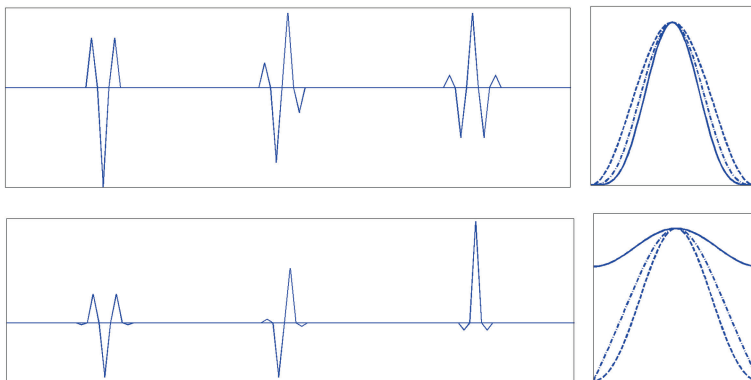
Fig. 17.3 Top left IRs of the analysis p-filters \mathbf{h}^1 for the semi-tight frames, which are defined in Eqs. left to right : (17.31) \longrightarrow (17.32) \longrightarrow (17.33). Bottom left IRs of the corresponding analysis p-filters \tilde{\mathbf{h}}^1 . Top right Magnitude responses of the synthesis p-filters \mathbf{h}^1 , which are defined in Eqs. (17.31) (dashed line), (17.32) (dash-dot line) and (17.33) (solid line). Bottom right Magnitude responses of the corresponding analysis p-filters \tilde{\mathbf{h}}^1
