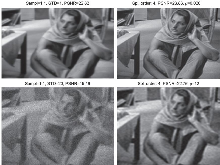
Fig. 7.9 Top left the blurred “Barbara” image corrupted by noise whose STD is 1, PSNR = 22.82 dB. Top right the cubic deconvolution spline, PSNR = 23.86 dB. Bottom left the image corrupted by noise, \sigma = 20 , PSNR = 19.46 dB. Bottom right the cubic deconvolution spline, PSNR = 22.76 dB
