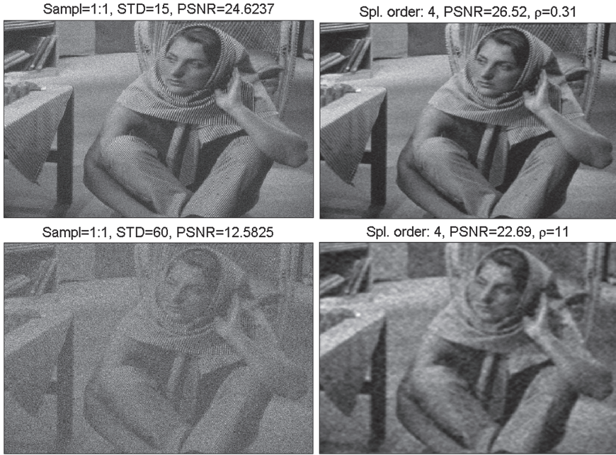
Fig. 13.7 Top left —“Barbara” image corrupted by noise whose STD \varepsilon = 15 , PSNR = 24.62 dB. Top right —cubic discrete smoothing spline, PSNR = 26.52 dB. Bottom left —the image corrupted by noise, \varepsilon = 60 , PSNR = 12.58 dB. Bottom right —cubic discrete smoothing spline, PSNR = 22.69 dB
