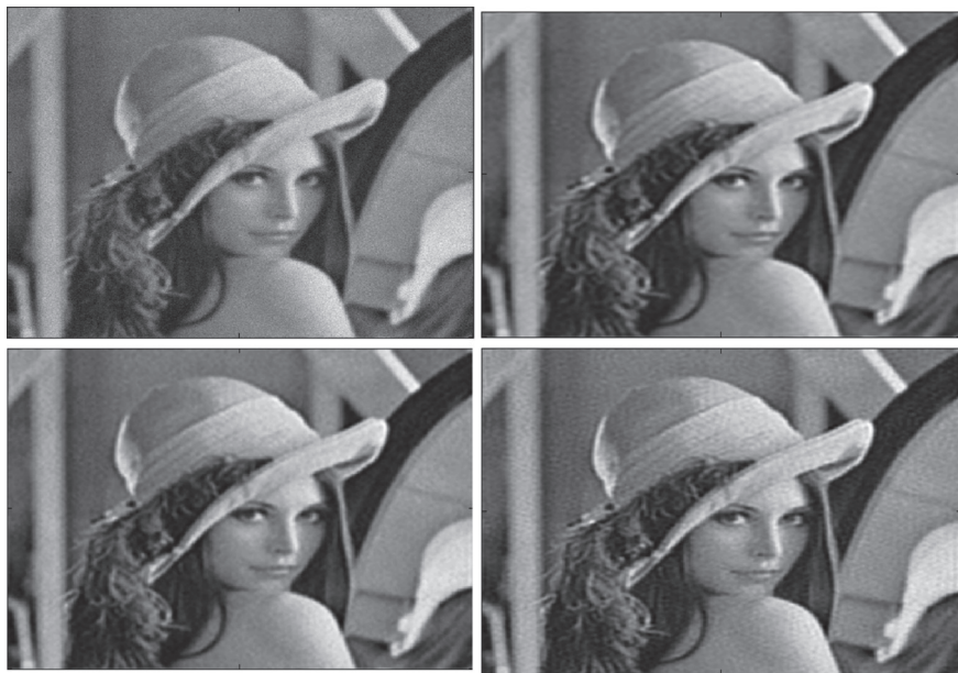
Fig. 11.6 “Lena”. Top left Blurred noisy image, t = 2 , noise STD = 10, PSNR = 25.15; Top right Image restored by GTA, PSNR = 27.93. Bottom left Image restored by BBA, PSNR = 28.20, spline wavelet packets of the fourth order from 6 levels were used, 600 waveforms were involved. Bottom right Image restored by BPA, PSNR = 28.29, spline wavelet packets of the fourth order from 6 levels were used. Number of best blocks per iteration B = 600 . The result is achieved by 2 iterations
