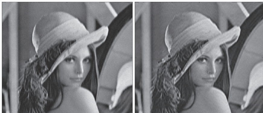
Fig. 14.20 Reconstruction of the “Lena” image from a blurred (Gaussian, \sigma = 3 ) and noised (STD = 5) input. Left input; Right restored image
