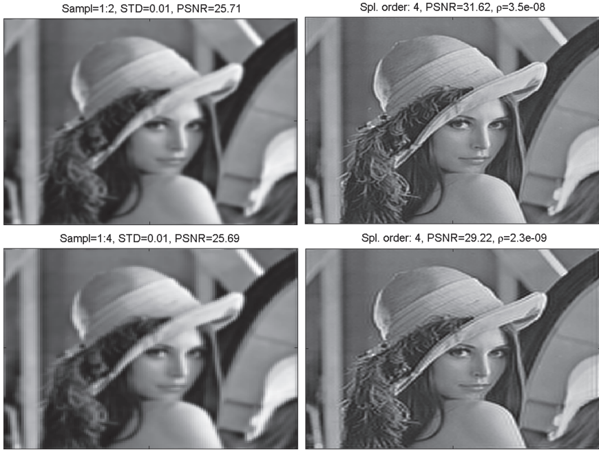
Fig. 7.11 Top left the blurred “Lena” image downsampled at 1:2, noise STD is 0.01, PSNR = 25.66 dB. Top right the cubic deconvolution spline, PSNR = 31.24 dB. Bottom left the image downsampled at 1:4, PSNR = 25.5 dB. Bottom right the cubic deconvolution spline, PSNR = 27.26 dB
