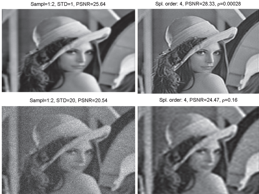
Fig. 7.10 Top left the blurred “Lena” image downsampled at 1:2 and corrupted by noise whose STD is 1, PSNR = 25.64 dB. Top right the cubic deconvolution spline, PSNR = 28.33 dB. Bottom left the image corrupted by noise, \varepsilon = 20 , PSNR = 20.54 dB. Bottom right cubic deconvolution spline, PSNR = 24.47 dB
