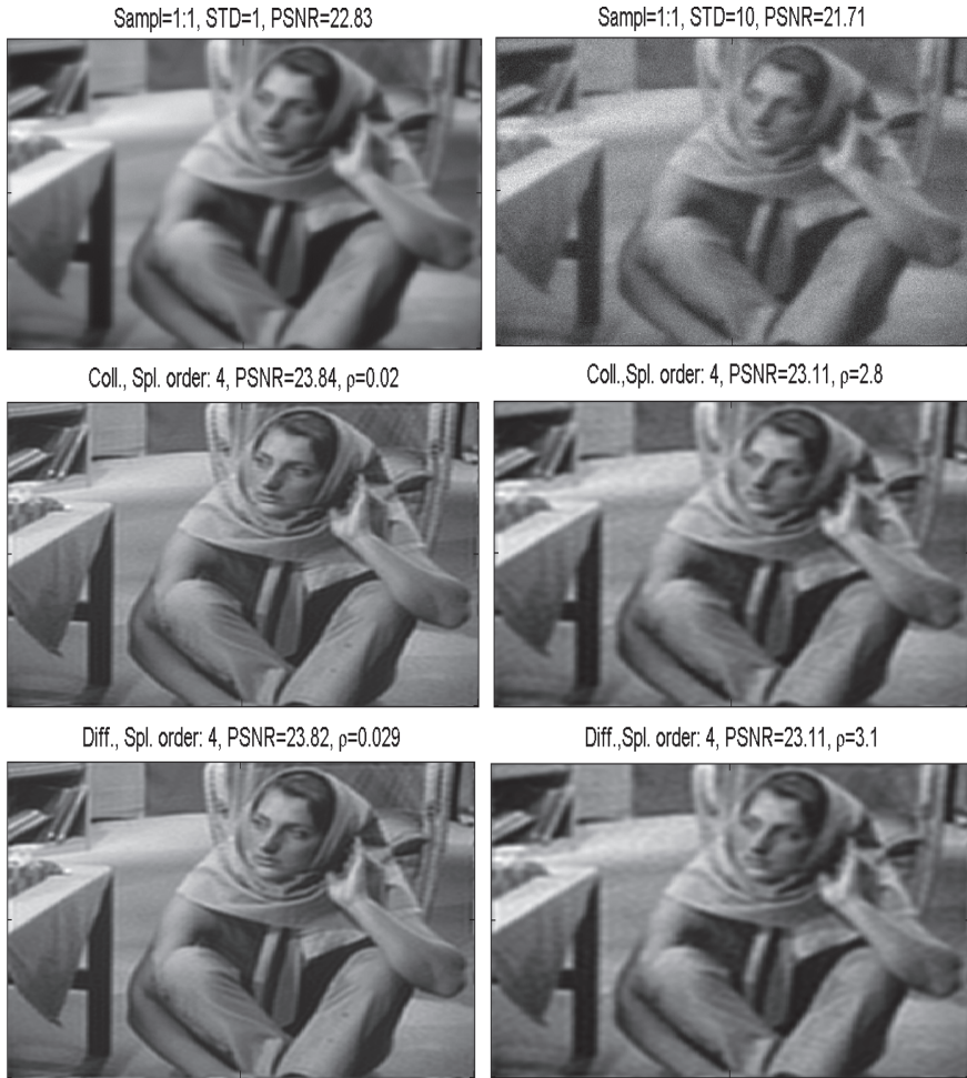
Fig. 7.16 Top left the blurred “Barbara” image ( t = 5 ) corrupted by noise whose STD is 1, PSNR = 22.83 dB. Top right the blurred “Barbara” image ( t = 5 ) corrupted by noise whose STD is 10, PSNR = 21.71 dB. Center left the image restored by the cubic spline S_\rho[\mathbf{z}, t](k, n) , PSNR = 23.84 dB (collocation approximation). Bottom left the same with the difference approximation, PSNR = 23.82 dB. Center right the image restored by the cubic spline S_\rho[\mathbf{z}, t](k, n) , PSNR = 23.11 dB (collocation approximation). Bottom right the same with the difference approximation, PSNR = 23.11 dB
