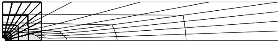
Fig. 3.21 Stretched geometry of a rectangular sheet with a hole
