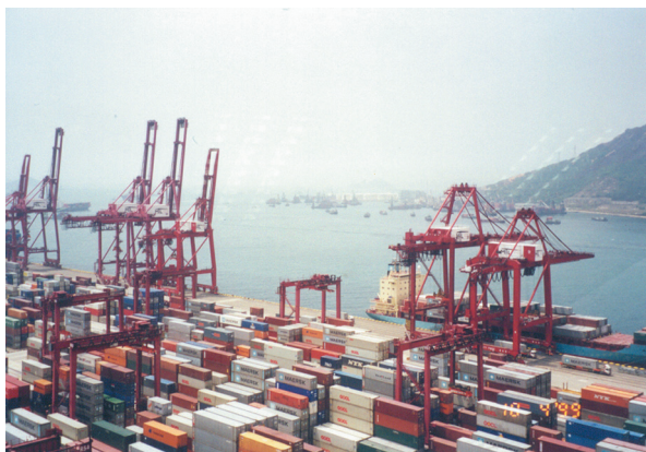
Fig. 1.4 Containers in temporary storage at the storage yard (SY). At water's edge, see quay cranes (QCs) unloading import containers (ICs) from, and loading export containers (ECs) into, vessels. In SYs see yard cranes (YCs) that store and retrieve containers from storage
