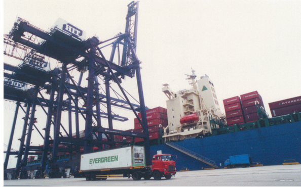
Fig. 1.3 A docked container vessel and quay cranes (QCs) unloading inbound containers (ICs) from it and loading outbound containers into it. Also see an internal truck (IT) (that transports containers between the berth and the storage yard (SY)) loaded with an IC that it is taking to the SY
