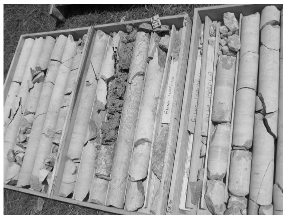
Fig. 13 A karst cave (an empty core of the T 1-8 borehole) at the depth of 217.2–220 m
