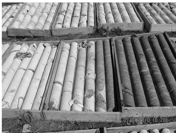
Fig. 17 A part of the core from the T 2-13 borehole that shows a tectonic overthrust transition from limestone ( lighter cores ) to flysch ( darker cores )
