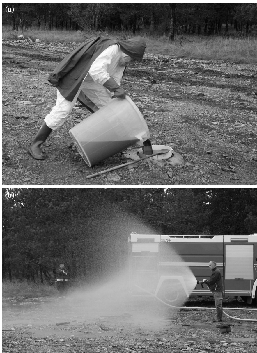
Fig. 14 Injection of uranine into the T 2–12 borehole (a) and spray irrigation of the surface near the borehole (b)
