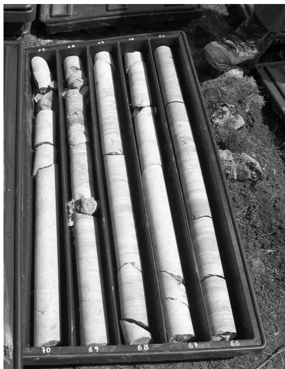
Fig. 15 Flowstone is located at the depth between 68.1 and 68.7 m and fills up the karst cave in the T 2-9 borehole
