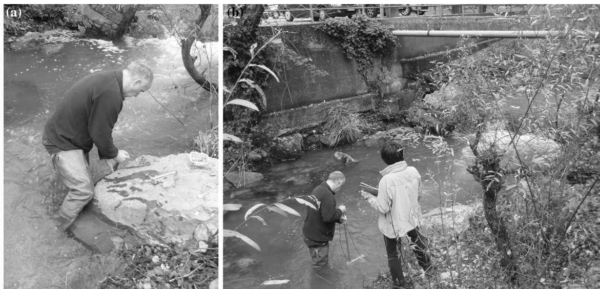
Fig. 7 Placement of the water level data logger at the common flow of the Boljunec springs (a) and measurement of the total discharge with the current meter (b)
