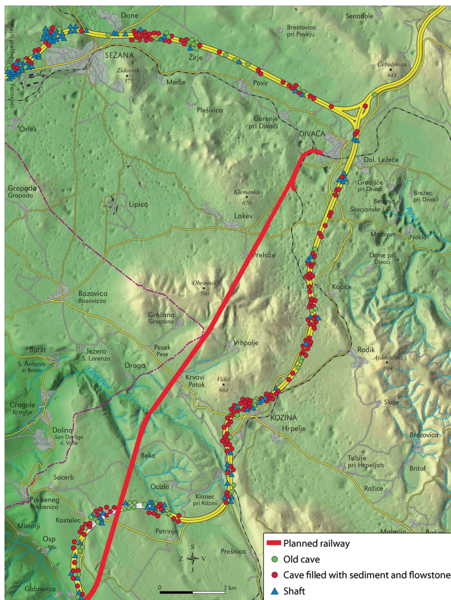
Fig. 4 Caves which opened up during the construction of the motorway between Divača, Fernetiči and Črni Kal, and the planned railway line (from Knez and Slabe 2007)
