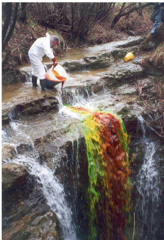
Fig. 9 Injection of uranine into a stream that sinks into the Beka-Ocizla cave system
