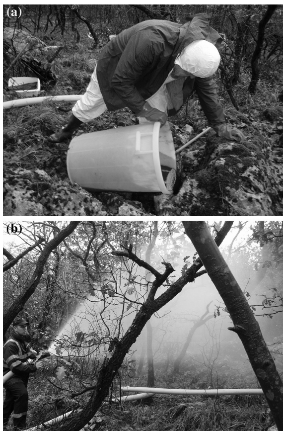
Fig. 11 Injection of uranine into a fissure near the Črnotiče quarry (a) and additional spray irrigation of the injection spot (b)
