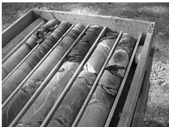
Fig. 14 Lithological changes in flysch as seen in the core of the T 1-11 borehole
