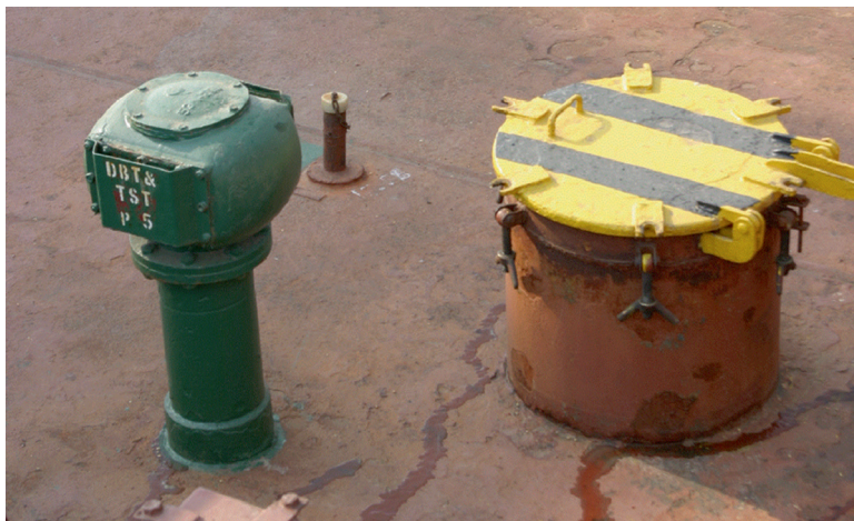
Fig. 6 An air-vent on the left , a sounding pipe in the center back , and a TST hatch on the right on a bulk carrier
