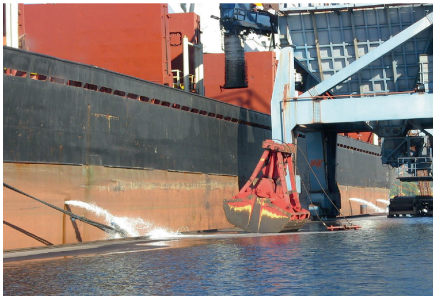
Fig. 2 Ballast water discharge above pier level from the upper wing tanks of a bulk carrier (Photo: Jure Barovič, Port of Koper)
