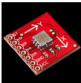
Accelerometer to measure tilt angle
