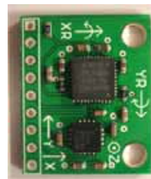
Gyro to measure the angular velocity
