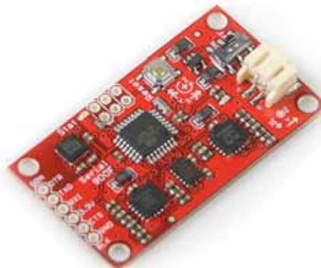
IMU: Inertia Measurement Unit
