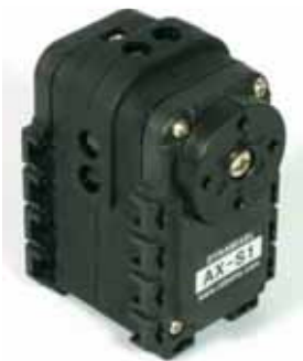
AX-S1 (Integrated Sensor Module Includes: 3 IR sensors, Remote control sensor, Microphone, Buzzer)
